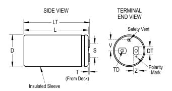
**General Information** Series ALS30 Dielectric Aluminum Electrolytic Description Screw Terminal, Aluminum Electrolytic RoHS AEC-Q200 No Typical Component 220 g Weight Dimensions D And L Include Sleeving. MS (MxH) = M12x16. Mounting Clamp (Sold Separately): Notes V4/2737 Shelf Life 156 Weeks
