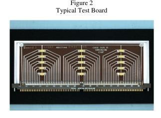
Test conditions were selected after consultation with the supplier and some internal consultation. It was decided to perform life test on an increased sample size at rated voltage and 105°C (although testing is usually performed at 85°C and 125°C). A scanner was used to monitor each part once a minute and fuses were selected to blow at 590 ma.
