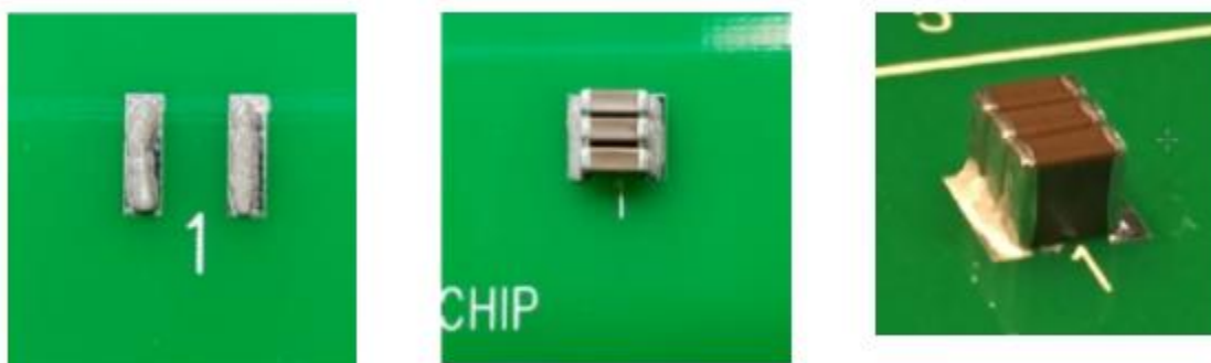
Figure 5 – Solder Paste on KONNEKT 1812 Land Patterns
