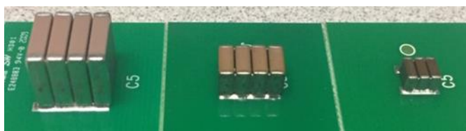
Figure 3 - KONNEKT Capacitors mounted in Low-Loss Orientation. From left to right: 3640 4-chip, 2220 4-chip, 1812 4-chip
