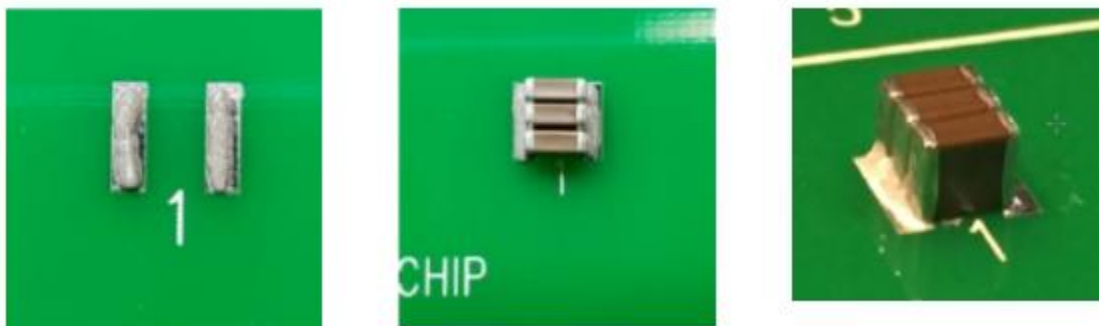
Figure 5 – Solder Paste on KONNEKT 1812 Land Patterns
