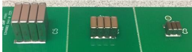
Figure 3 - KONNEKT Capacitors mounted in Low-Loss Orientation. From left to right: 3640 4-chip, 2220 4-chip, 1812 4-chip
