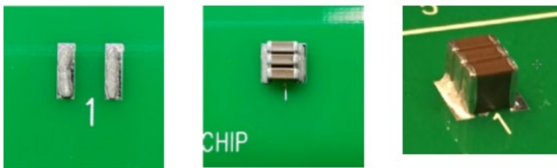
Figure 6 – Solder Paste on KONNEKT 1812 Land Patterns
