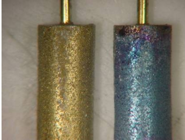
Fig. 1. Virgin (left) and failed (right) anodes of the A-case 22 uF – 25 V Wet Ta capacitors subjected to 200° C life test.
