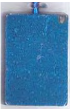
Figure 4. Picture of Stripped Capacitor Revealing Failure Site at Top Edge of Anode
