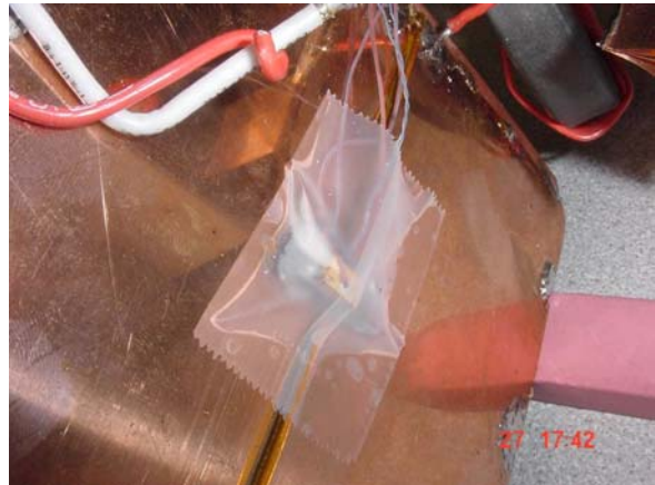
Figure 6. Close-up of Capacitor Soldered to Negative and Positive Heat Sinks. Capacitor is Covered with Thin Plastic Tape to Minimize Heat Dissipation via Convection.
