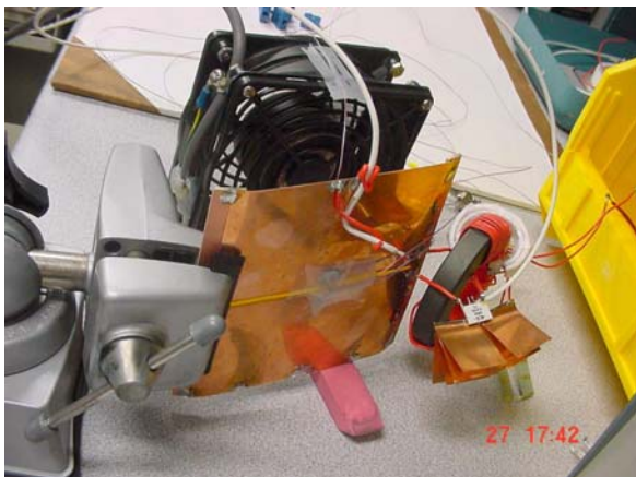
Figure 5. Detailed View of Fan, Capacitor on Split Heat Sink, Support Vise, Matching Transformer, and Current Sense Resistor with Fins.
