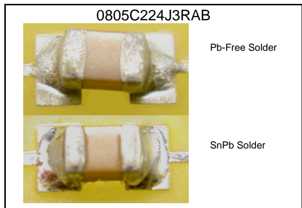
Figure 12. Solder fillet difference.
