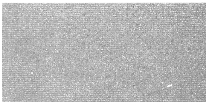
Figure 6. DPA of MLCC with no defect.
