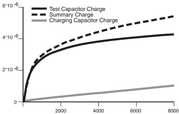
Figure 2. Charge (Q) vs DC Bias
