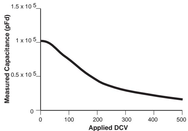
Figure 1. Capacitance vs DC Bias for Typical X7R Capacitor
