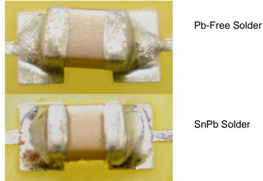
**Figure 12. Solder Fillets**
