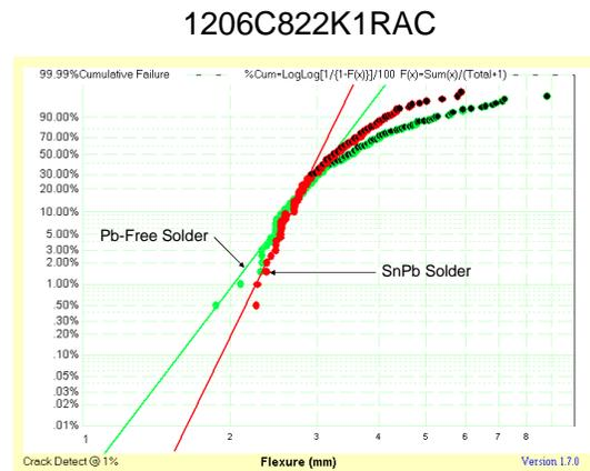
**Figure 8. Flex performance 1206, 8.2 nF X7R, Pb-Free vs. SnPb Solders**
