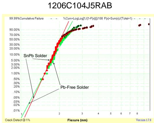
**Figure 9. Flex performance 1206, .1 uF X7R, Pb-Free vs. SnPb Solders**
