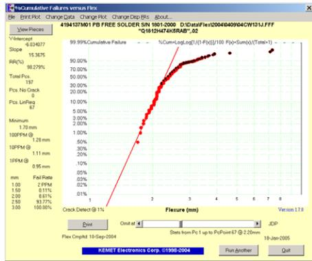
**Figure 2. Weibull plot of 1812, .47 uF, X7R**
