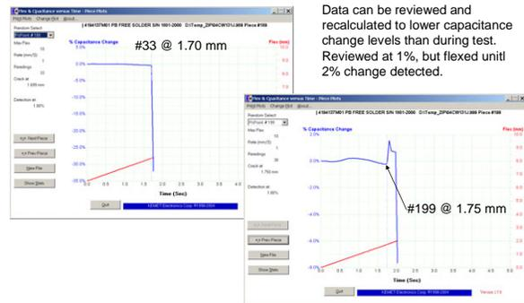
**Figure 4. Actual data for the two lowest readings.**
