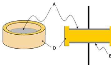
Figure 2. “Doorknob” structure for ceramic high voltage.
