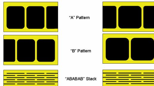
Figure 12. Five and four cascade electrode patterns.
