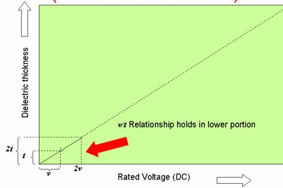
**Figure 5.** Voltage capability vs. thickness\_ low voltage.
