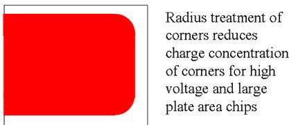
Figure 9. Reducing corner effect with radiused corners.
