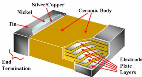
**Figure 4.** Multilayer ceramic chip structure.
