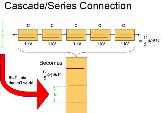
Figure 11. Five cascade vs. one of higher voltage.
