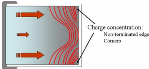
Figure 8. Charge concentration on one plate in MLC.
