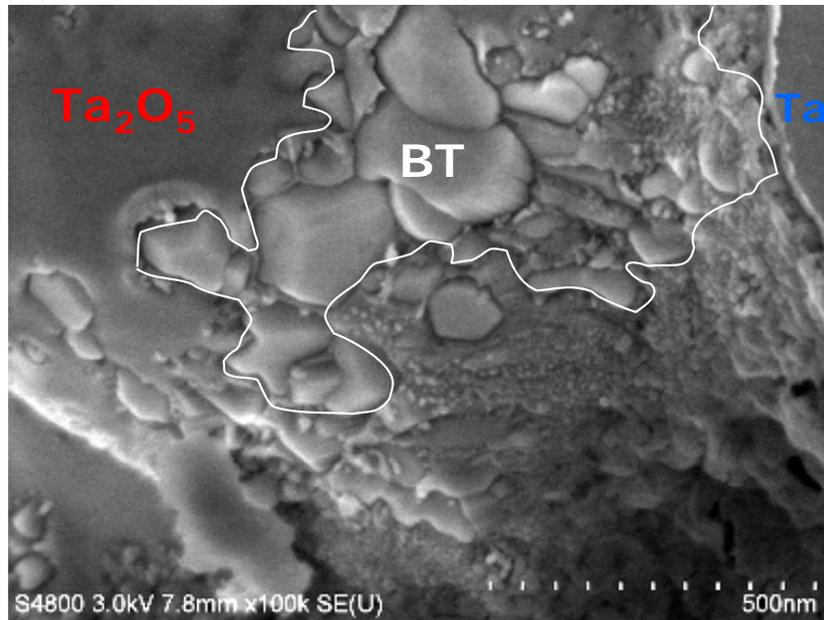
**Figure 10. Hybrid tantalum barium titanate capacitor structure**
