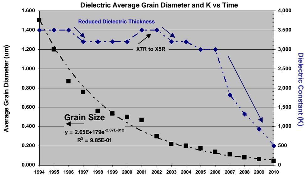
Figure 7. Evolution and projection of grain size and K for class 2 dielectric vs. time
