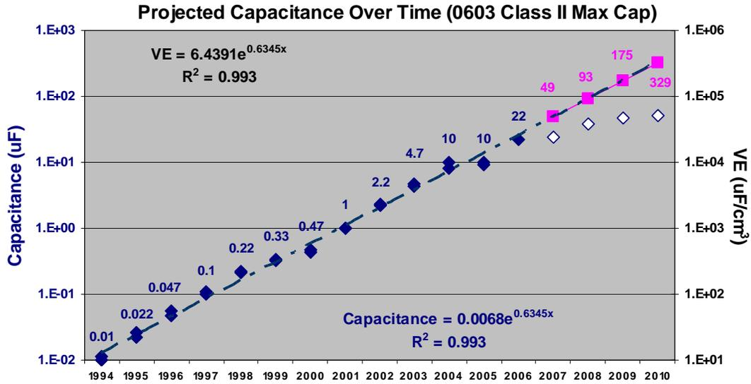
Figure 1. Evolution and projection of capacitance and VE with time, 0603 class 2 MLCC
