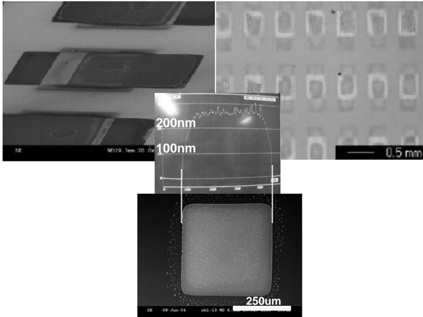
**Figure 12. MLCC produced via micropad stamping of a BaTiO<sub>3</sub> precursor solution at Penn State University**
