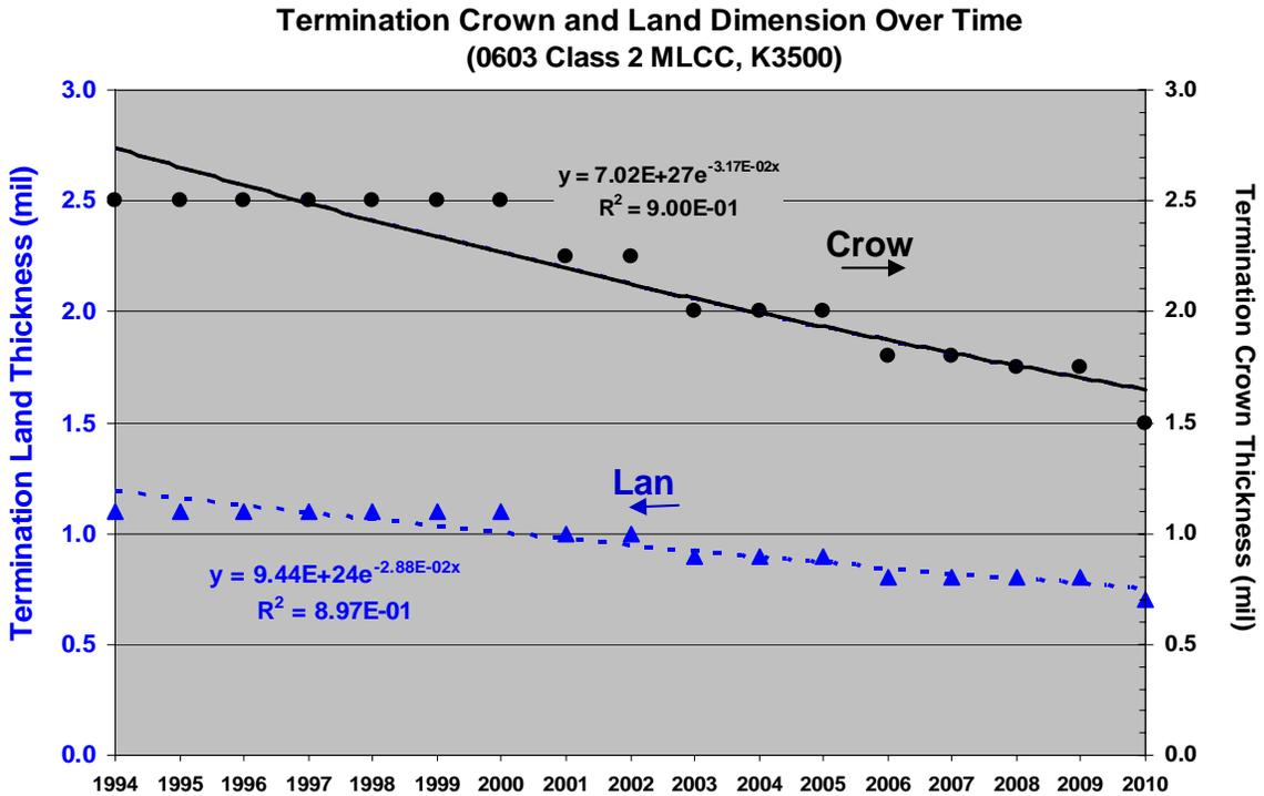
Figure 4. Evolution and projection of termination dimensions over time, 0603 class 2 MLCC
