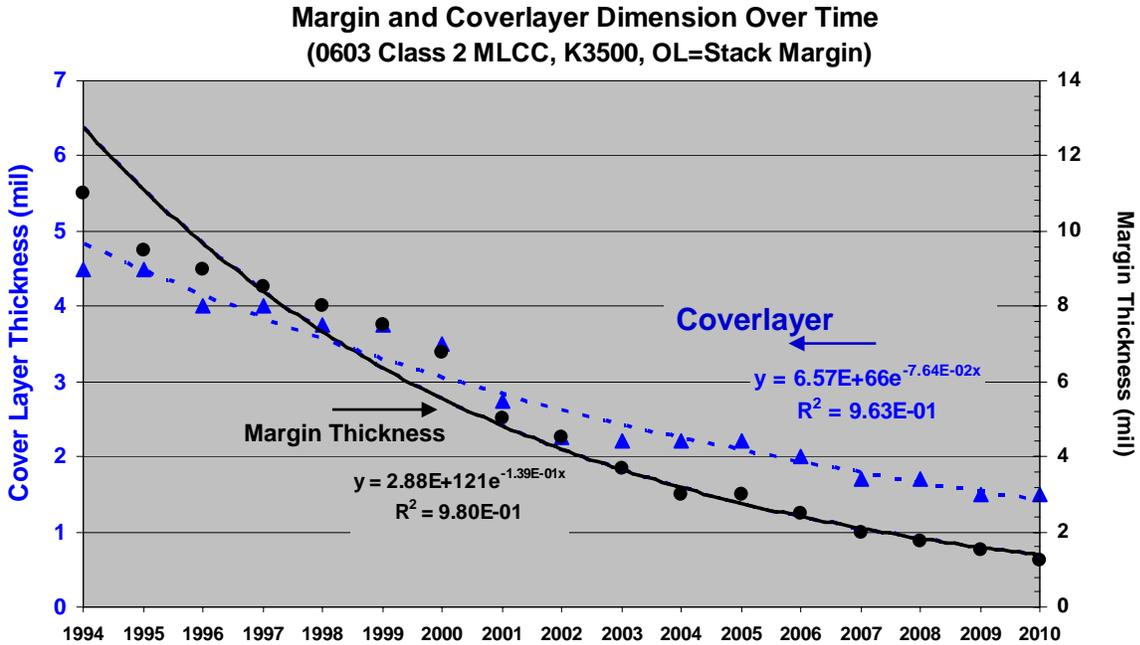
Figure 3. Evolution and projection of cover layer and margin dimensions with time, 0603 class 2 MLCC
