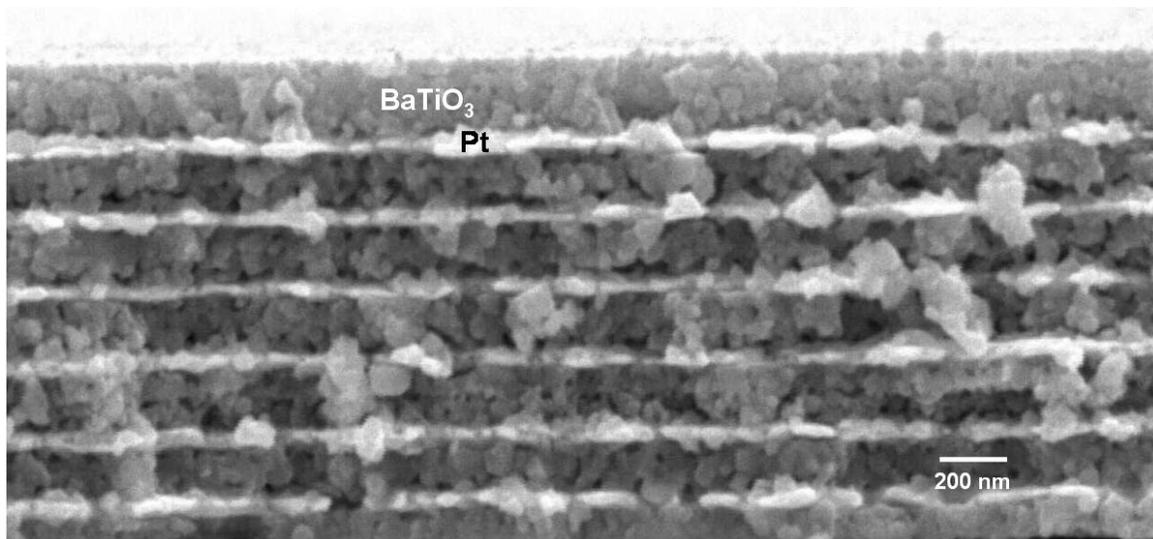
Figure 8. Thin film multilayer structure fabricated at Penn State University
