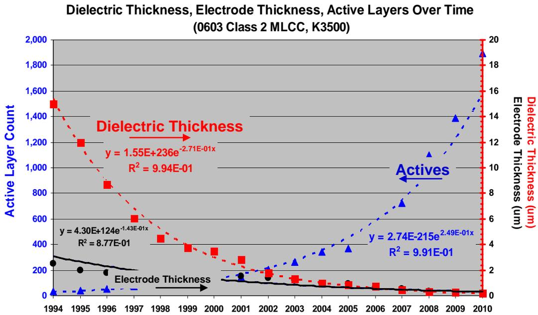
Figure 2. Evolution and projection of dielectric thickness, electrode thickness and active layer count over time 0603 class 2 MLCC
