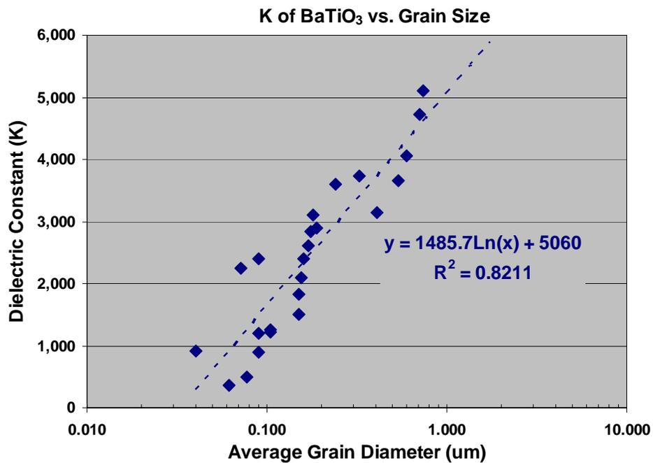
Figure 6. K of BaTiO<sub>3</sub> vs. average grain diameter<sup>5</sup>
