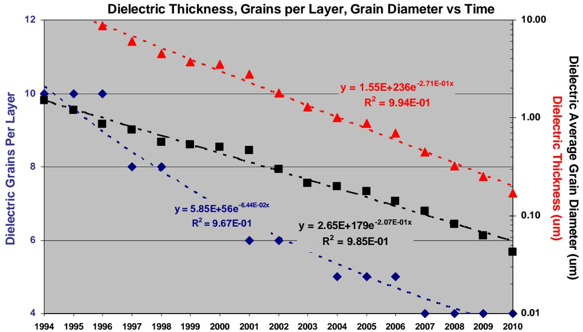
Figure 5. Evolution and projection of dielectric thickness, number of grains per layer and average grain diameter vs. time
