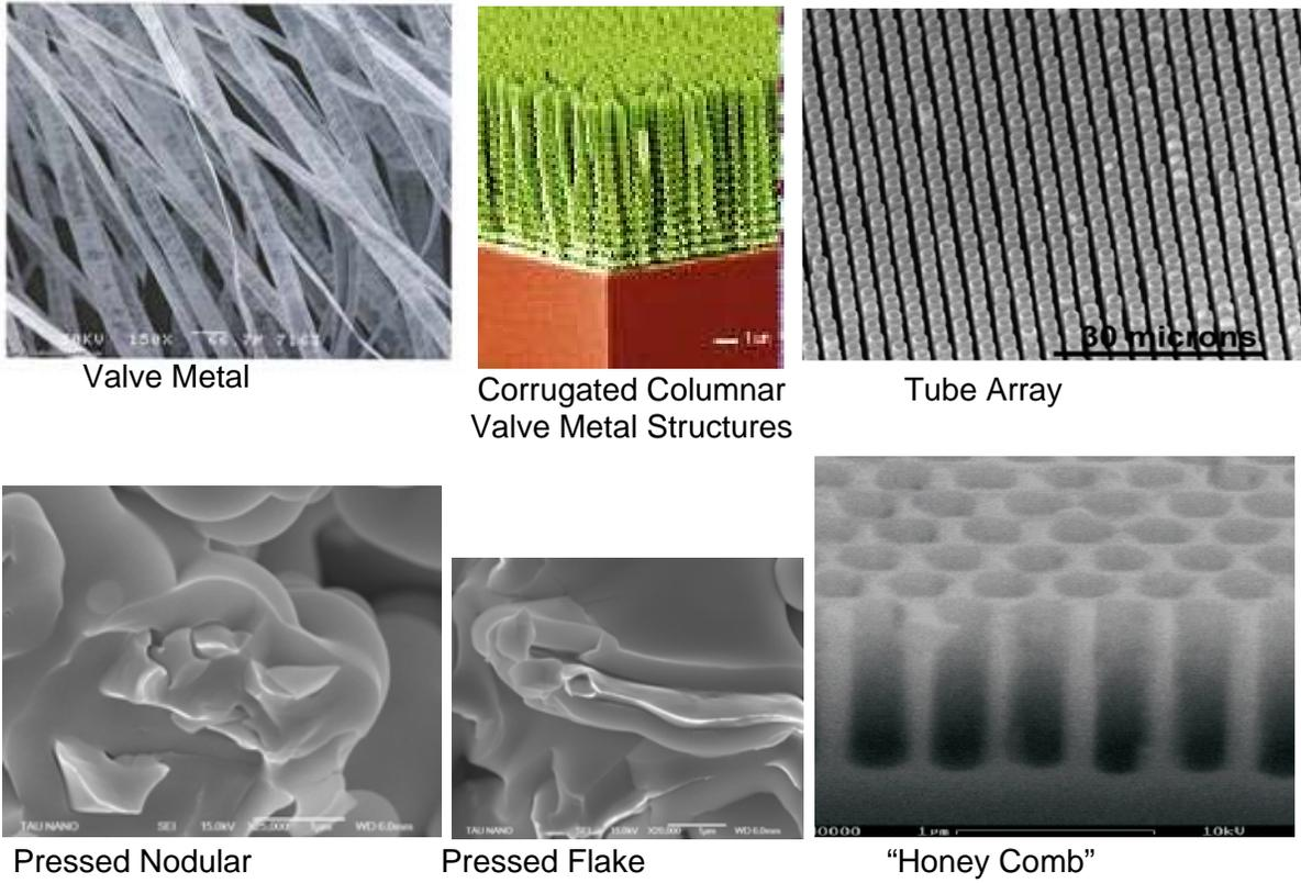
**Figure 11. Porous microstructures targeted toward maximizing surface area per unit volume in an open pore structure**
