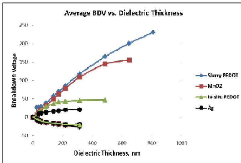
Fig. 1. Breakdown voltage as a function of the dielectric thickness [7].
