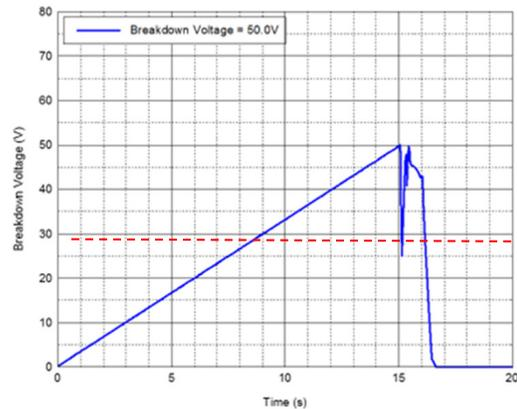
Fig. 6. Breakdown test data for PHS Ta capacitor with formation voltage 28 V
