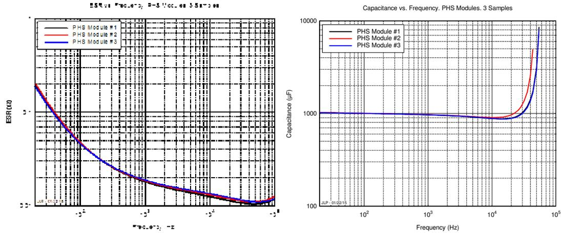
Fig. 5. ESR (left) and capacitance (right) frequency scans for 1 mF – 60 V modules with PHS Ta capacitors.
