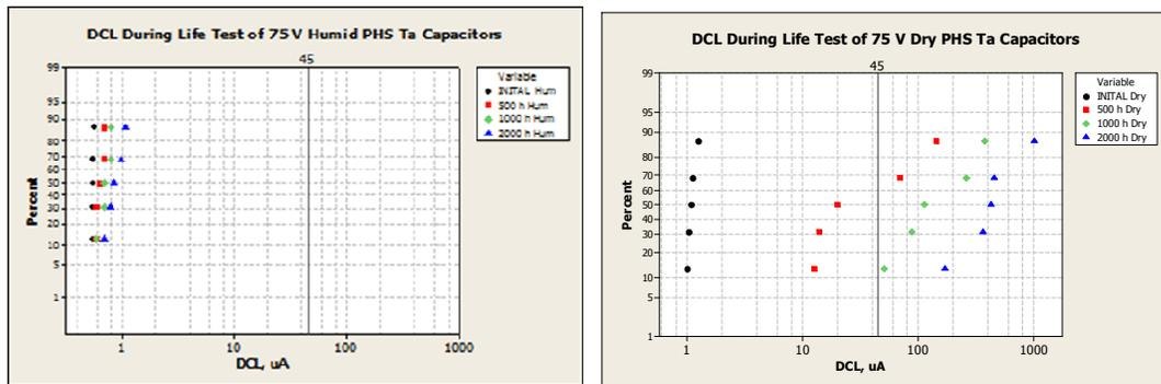
Fig. 2. DCL distribution during Life test in 75 V PHS Ta capacitors with moisture (left) and dry (right) [9].
