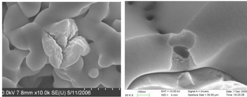
*Figure 1. The traditional process of fabricating the tantalum anode material resulted in cracks and pores.*
