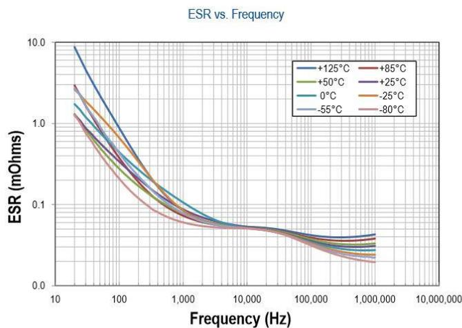
Figure 3. The T550 series maintains its low ESR over a wide range of temperatures and frequencies.
