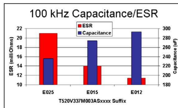
Figure 3. Relationship between capacitance and ESR.
