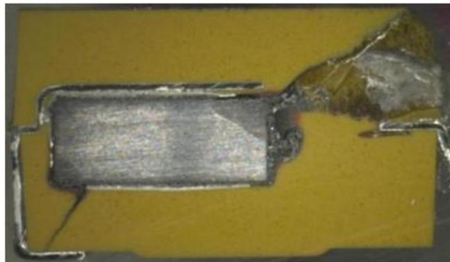
**Fig. 2. Cross-section of the failed Ta/MnO<sub>2</sub> capacitor**
