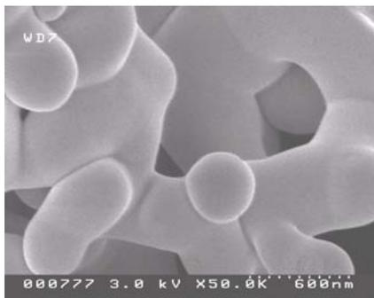
**Fig. 7. SEM images of Ta<sub>2</sub>O<sub>5</sub> dielectric formed on Ta anode manufactured with F1 technology.**
