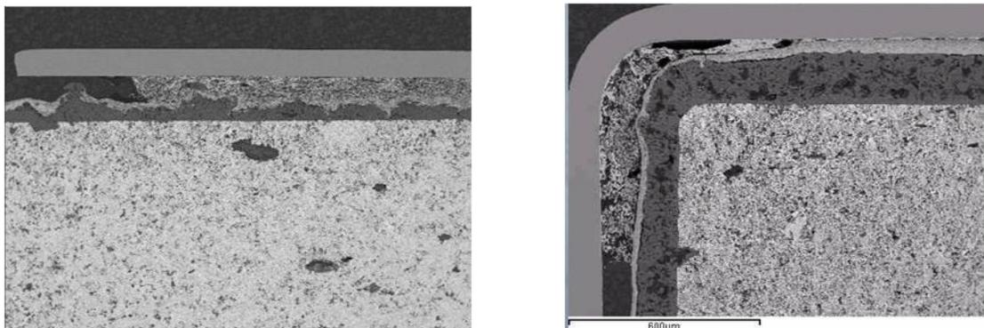
**Fig. 13. Cross sections of the Ta/MnO<sub>2</sub> capacitors 4.7 uF – 50 V from the two batches shown on Fig. 12.**
