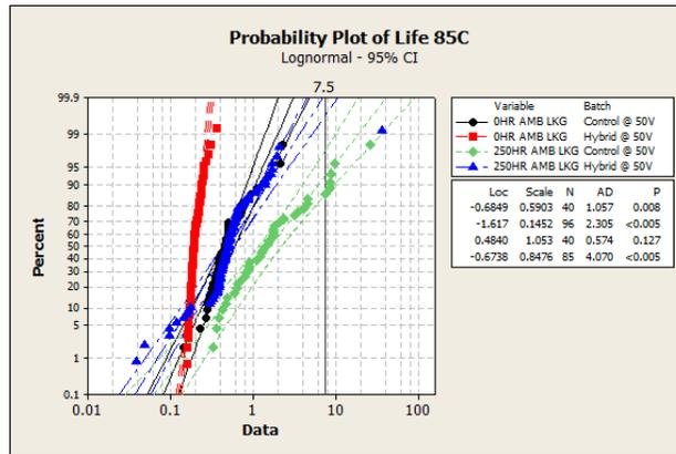
**Fig. 4. DCL distribution before and after 250 h Life test at 50 V and 85° C in Ta/MnO<sub>2</sub> capacitors with V<sub>f</sub> = 110 V (hybrid) and V<sub>f</sub> = 180 V (control)**
