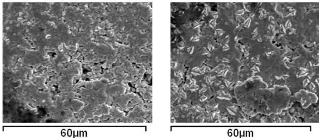
**Fig. 3. SEM images of the Ta<sub>2</sub>O<sub>5</sub> films with  $V_f = 110 \text{ V}$  (left) and  $V_f = 180 \text{ V}$  (right)**
