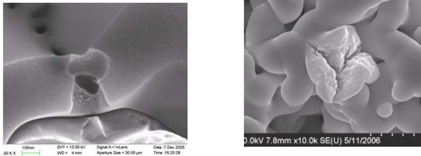
**Fig. 6. Ta<sub>2</sub>O<sub>5</sub> dielectrics formed on Ta surface enriched with carbon (left) and oxygen (right)**
