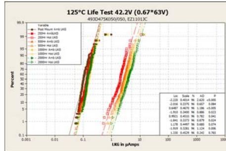
**Fig. 11. Room temperature and hot DCL in 50 V Ta/MnO<sub>2</sub> capacitors with F1 and SBDS tested as 63 V capacitors.**
