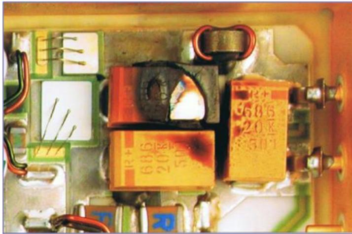
**Fig. 1. Failed Ta/MnO<sub>2</sub> capacitor on a circuit board**
