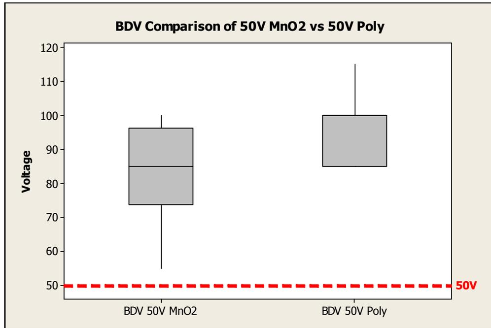
**Figure 1:** BDV Comparison of 50V MnO<sub>2</sub> and 50V Polymer Designs
