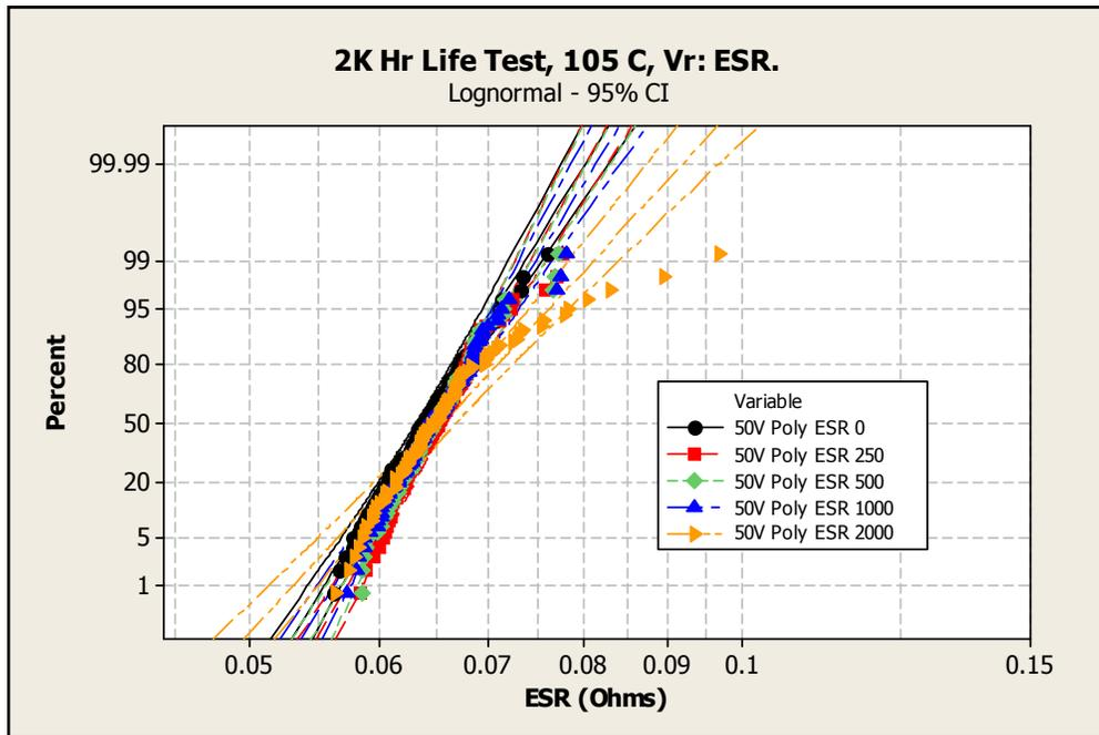
**Figure 4:** 50V Polymer Post 2000 Hours Life Test ESR Performance.
