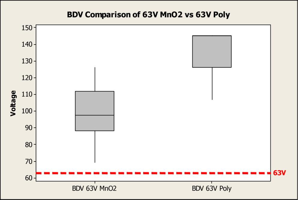
**Figure 2:** BDV Comparison of 63V MnO<sub>2</sub> and 63V Polymer Designs
