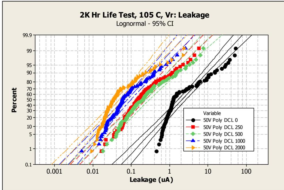
**Figure 5:** 50V Polymer Post 2000 Hours Life Test Leakage Performance
