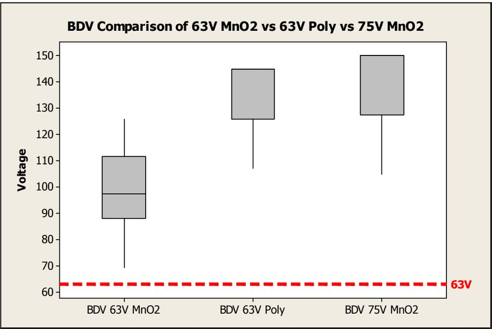
**Figure 3:** BDV Comparison of 63V MnO<sub>2</sub>, 63V Polymer and 75V MnO<sub>2</sub> Designs
