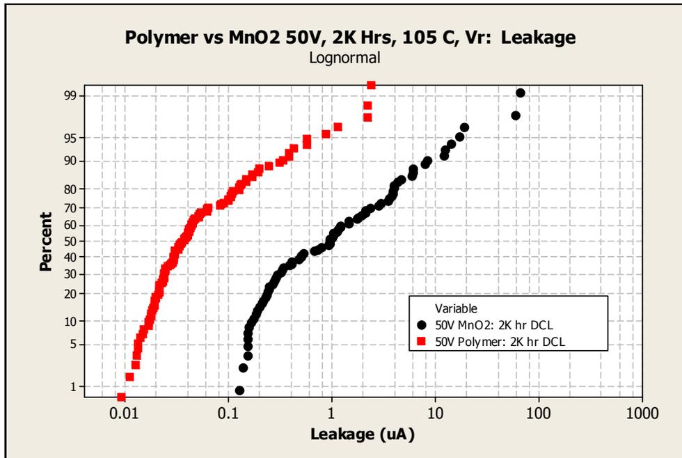
**Figure 6:** Leakage Performance of Polymer vs MnO<sub>2</sub> Tantalum Post 2000 Hrs Life Test
