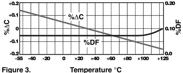
**Figure 3. Capacitance & DF vs Temperature - C0G**
