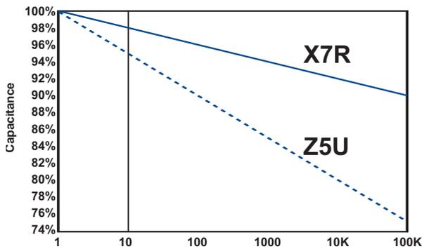
Figure 13. Typical Aging Rates for X7R & Z5U
