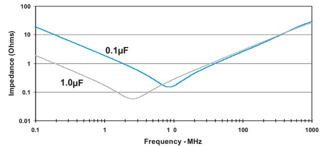
Figure 12. Impedance vs Frequency
