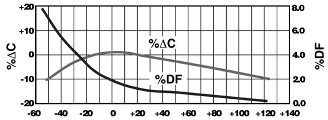
**Figure 4. Capacitance & DF vs Temperature - X7R**
