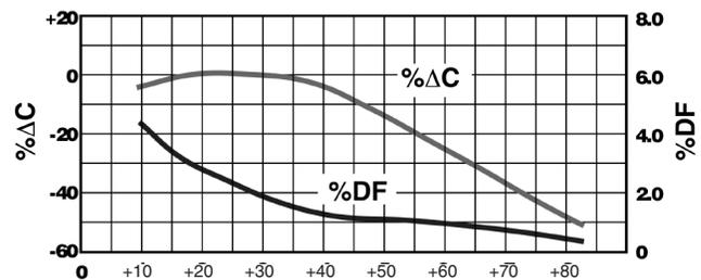
**Figure 5. Capacitance & DF vs Temperature - Z5U**
