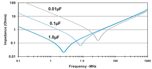
Figure 11. Impedance vs Frequency
