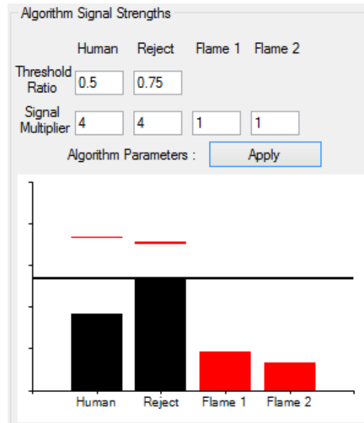
Figure 19 – Reduced Threshold Ratios and Increased Rejection Channel Multipliers
